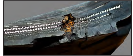
Improper tire repair.
